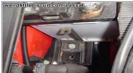
Once you have removed both the cables from the battery you will be faced with this which clamps the battery in place.
