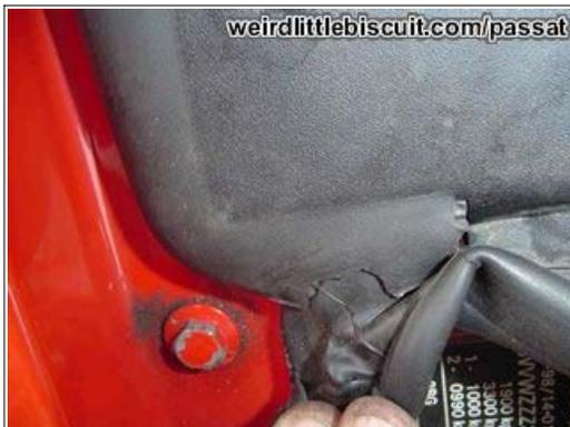
Nearly done, the final job to do in the engine compartment is to replace the seal around the engine and battery cover. Start at a corner and make sure that the rubber is pushed in tight. Also check that the battery cover is slotted correctly into the seal. Work your way round pushing it on firmly. Mine squeaked like a fat man on leather sofa, so if you hear that your doing it right.
