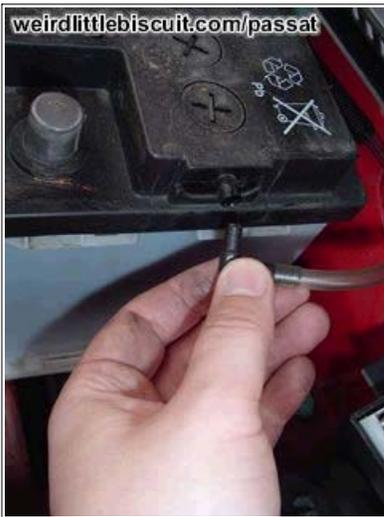
Wouldn't life be nice and simple if the battery just lifted out at this point. Well life isn't and it doesn't :) This little hose at the right a hand side for run off from the battery just pulls out.
