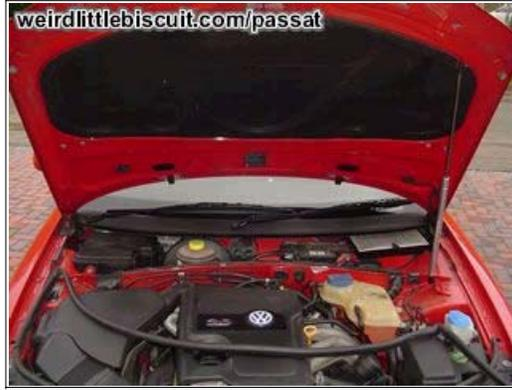
The first thing you need to do is remove the seal that runs around the edge of the engine to remove the battery cover. The rubber seal just pulls off and the cover just slides out by pulling it towards the front of the car. You should be left with something similar to the image below.
