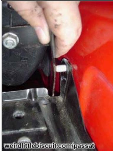
Now the shelf the battery was sitting on needs to be removed. It is held in place with two nuts and a bolt. This image shows the top left of the shelf with the nut removed. This one nut holds the alarm sounder (that's what it looks like to me anyway) in place as well as securing the shelf to the body. The alarm sounder and the shelf slot together so they have to be unslotted. With all the fixings removed and the alarm sounder out of the way the shelf just lifts out.
