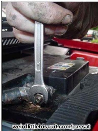
There are two drain holes and to get to them we need to remove the battery and the shelf it sits on, don't be frightened, its easy really. First off the battery needs to be removed using your trusty 10mm spanner mentioned earlier.
