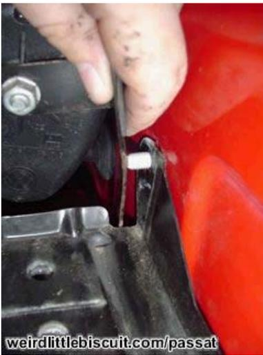
So with everything de-gunked its time to put everything back together. When reconnecting the battery shelf, remember to put the alarm sounder after the shelf is in place or it wont slot together properly.
