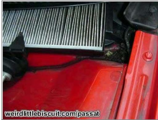
This is a close up of the [pollen filter which incidentally needs changed, but thats a job for another day](#). As you can see there is a line of sludge along the route the water run off should be taking. Over time its this sludge that blocks the drain holes. If your car dosen't have this sludge the drain holes could still be blocked. Might be worth looking into it anyway.
