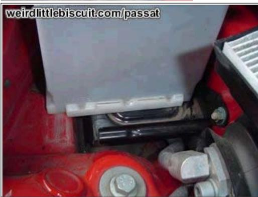
Slide the battery in place so that its hard up against the lip at the right hand side of the shelf.
