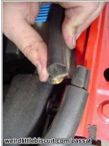
The seal that runs around the engine slots together at two points the left and right, make sure that these are properly slotted together.
