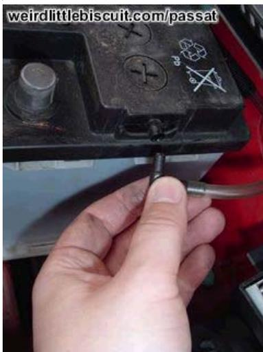
Re attach the battery run off hose at the right a hand side and check that the other end is pointing towards the newly unblocked drain hole.
