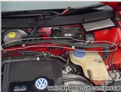
The cable marked here needs to be unclipped from the body of the car to allow you to remove the battery.
