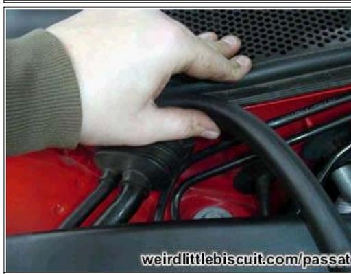
Replacing the seal starting in the top left corner.
