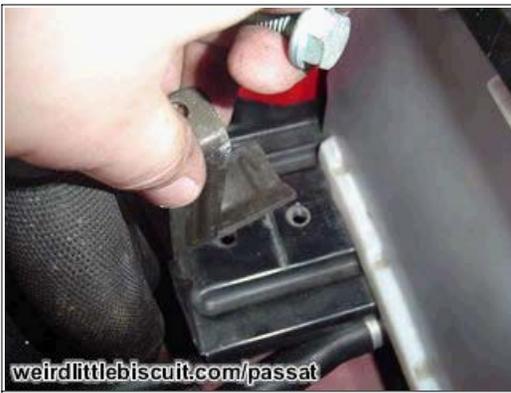
Using a 14mm socket remove the bolt and clamp which just lifts off.
