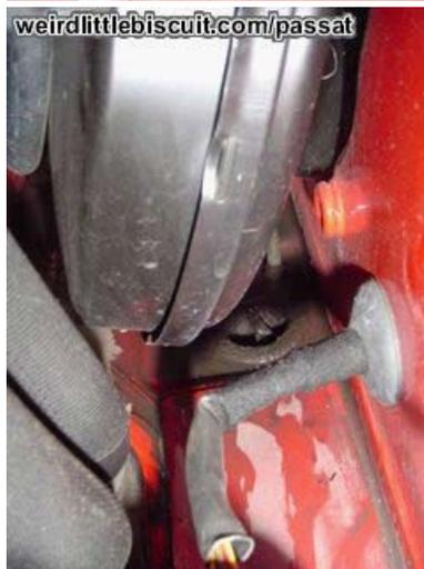
The big black thing you can see at the top left is the break master cylinder and under this you can see the second drain hole which is very gunked up with sludge.
