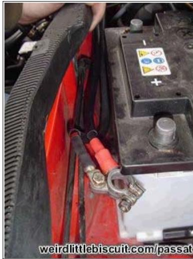
Before you replace the clip on cable shown here you need to make sure the cables you are going to attach to the battery are tucked in this space as shown here. They wont slot through with the larger cable clipped in place.
