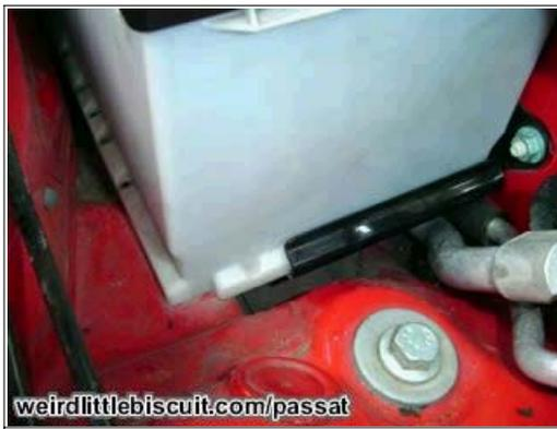
The shelf the battery sits on has a lip at the right hand side which, together with the clamp we removed earlier hold the batter in place. The battery needs to be slid to the left so it clears this lip then it simply lifts out. Remember though its bloody heavy and contains acid and other nasty stuff. modern batteries are sealed but its best to keep it level and treat it with a little respect just incase.
