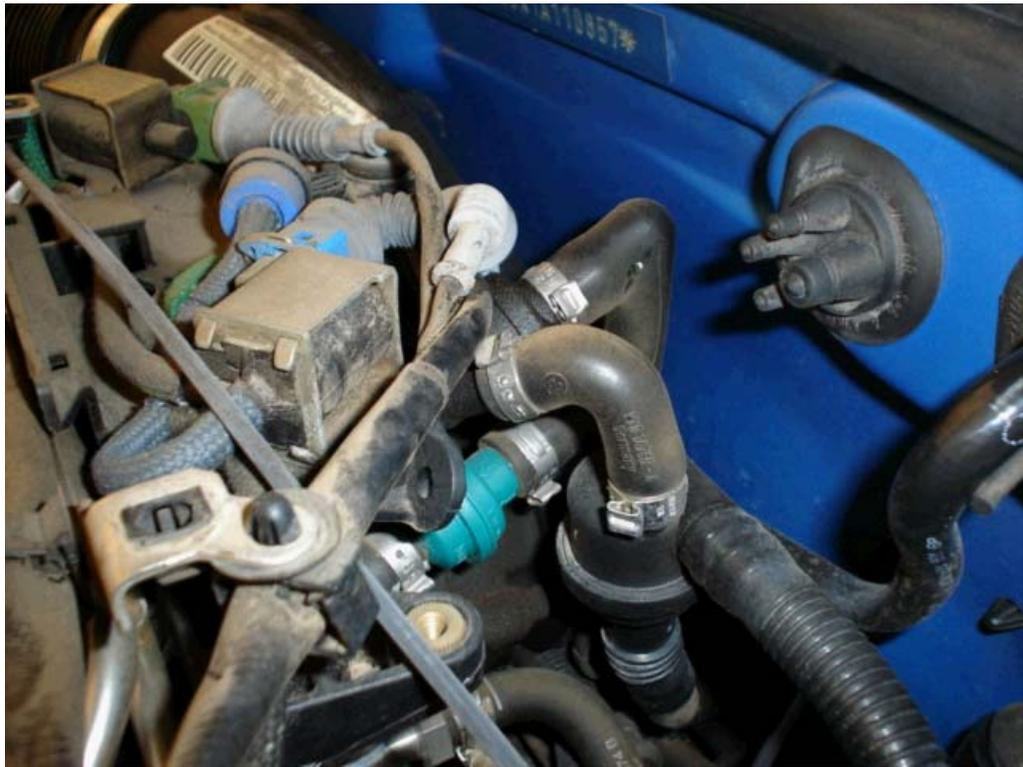
Cut the one time clamp off carefully, not to puncture the hose and remove...
