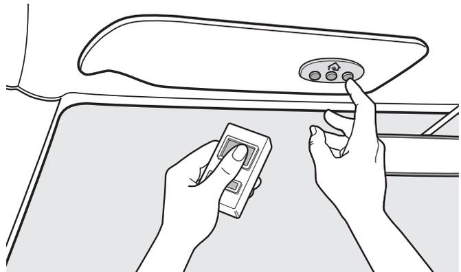
4. Hold down both buttons until the indicator light on the HomeLink Wireless Control System flashes, first slowly then rapidly. When the indicator light flashes rapidly, both buttons may be released. (The rapidly flashing light indicates successful programming of the new frequency signal.) To activate the garage door or other programmed device, press and hold the HomeLink button—releasing when the device begins to activate.
